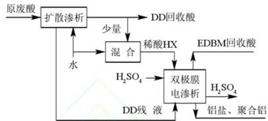
图 4 扩散渗析与双极膜电渗析技术联用于电极箔腐蚀零排放废酸回收处理工艺流程 Fig.4 Simplified flow diagram of the DD and EDBM coupled system for foil industry waste acid recovery
